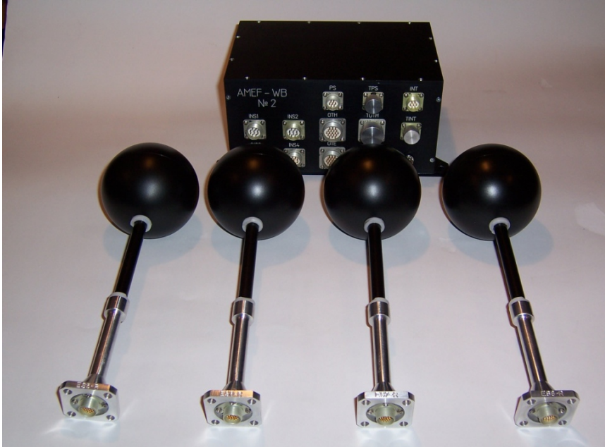
Fig. 4. Layout of the AMEF-WB/IESP-3R device and electric sensors
